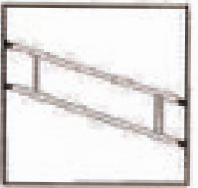
Guardrail double beam
